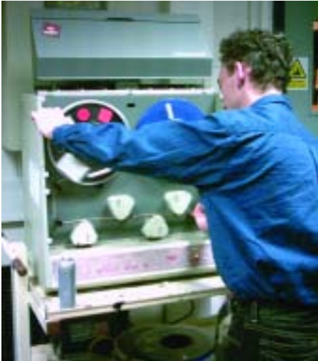
Dirty tapes are cleaned with tissue paper and a careful hand
